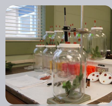
Fig 1A. Branch sealed in air-tight jar to incubate for 60mins for VTC extraction
