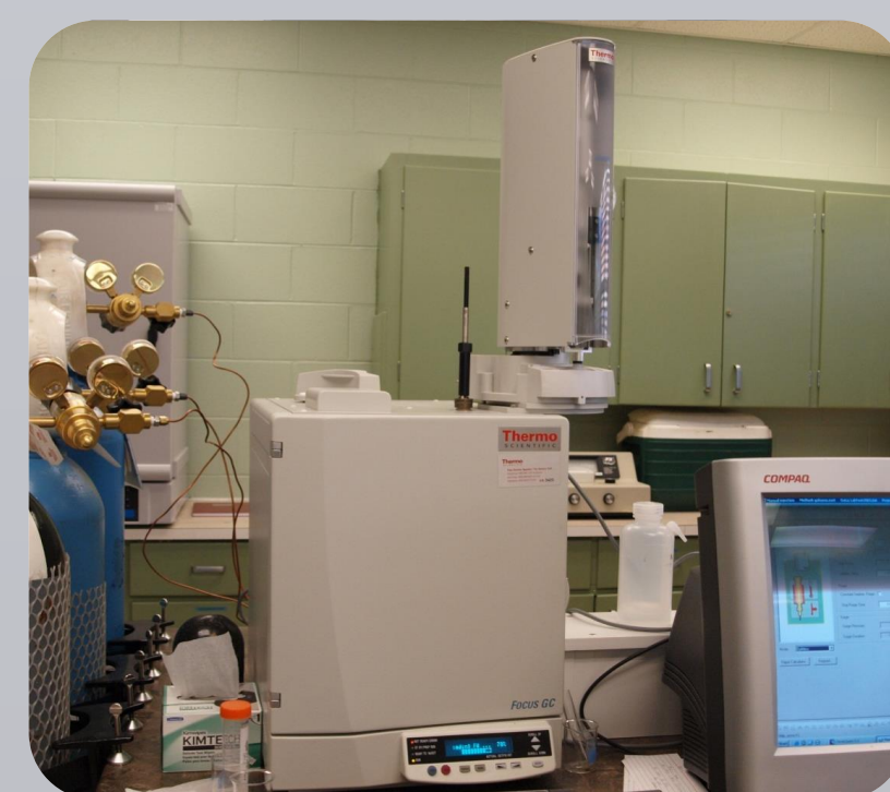
Fig 1C. VTC and ethylene analysis using GC-FID
