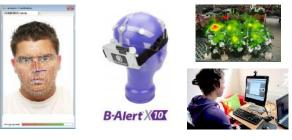
Discrete choice experiment will be combined with eye tracking technology and electromyographic (EMG) data to assess respondent's cognitive response to stimuli and electroencephalogram (EEG) to study brain activity while responding to the experiment stimuli.
