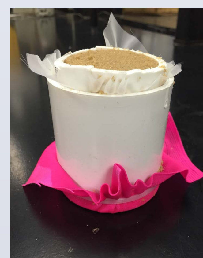
Fig 2: Ion exchange resin lysimeter used to measure mineral N leaching.
