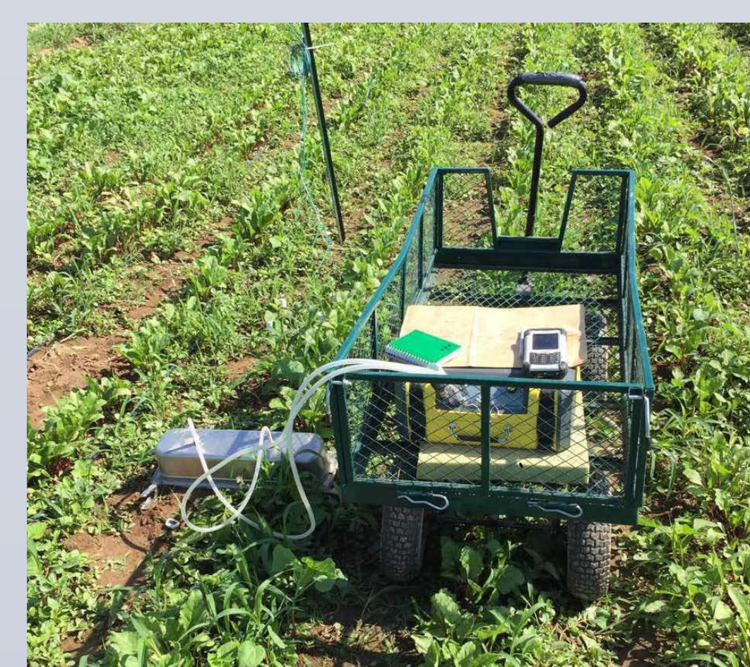
Fig 3: Gasetm DX4040 FTIR-based field gas analyzer used to measure trace gas fluxes.
