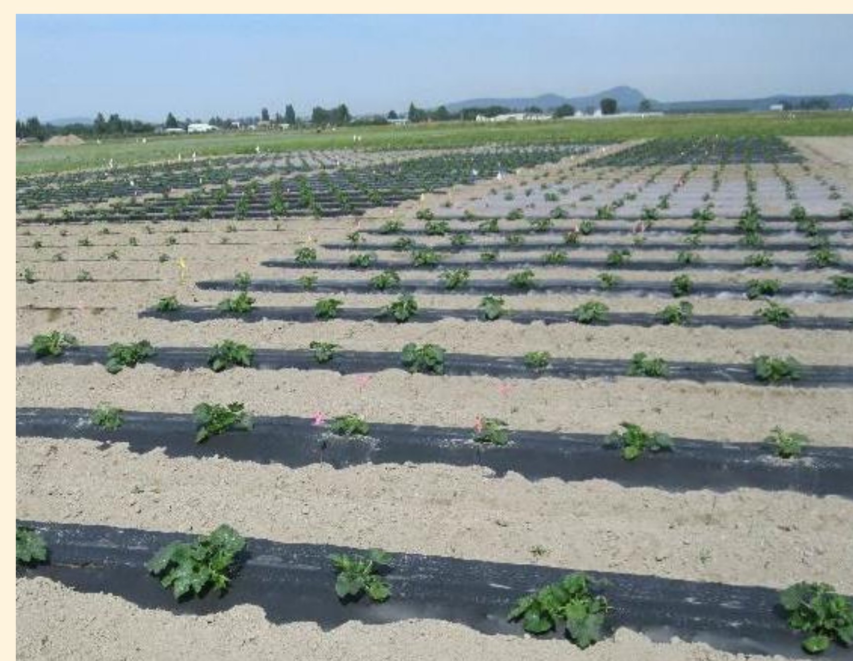
Fig. 2. Field experiment with 5 BDMs and 1 PE mulch at WSU Mount Vernon NWREC in 2015.
