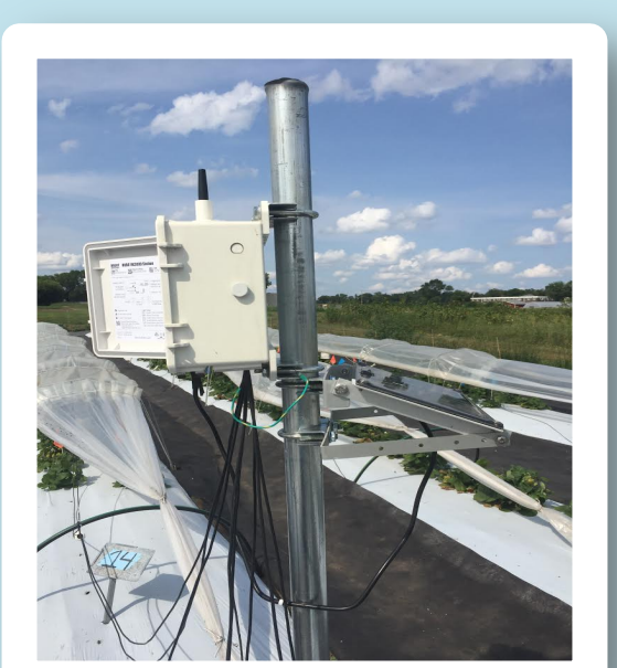
HOBO Onset RX3000 Remote Weather Station with sensors
