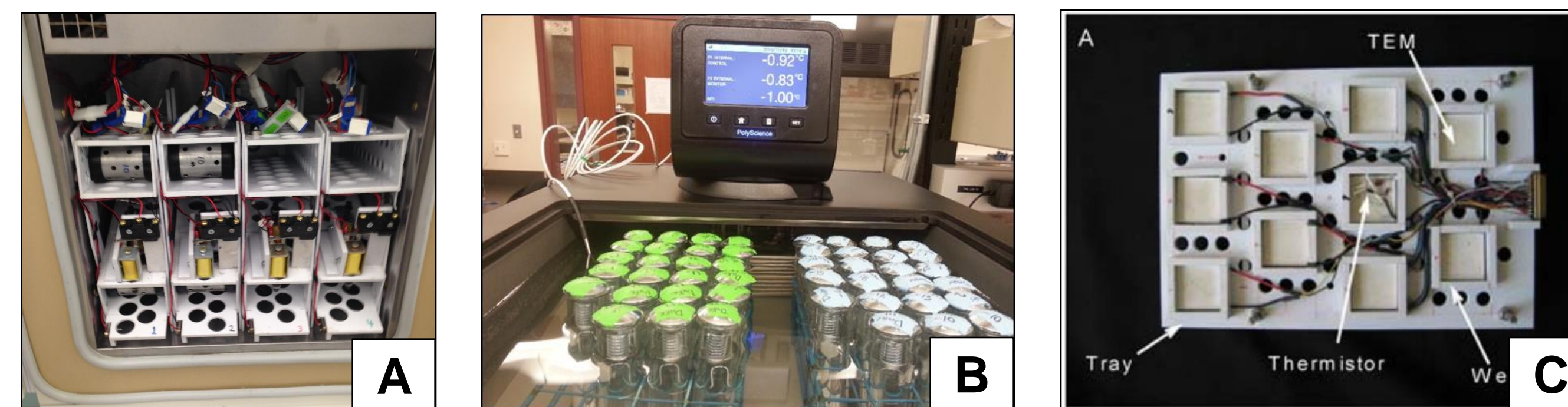
Figure 3. Equipment tested to determine an appropriate and reliable method to assess cold damage in blueberry include a programmable freezer (A), glycol bath (B), and differential thermal analysis (C).
