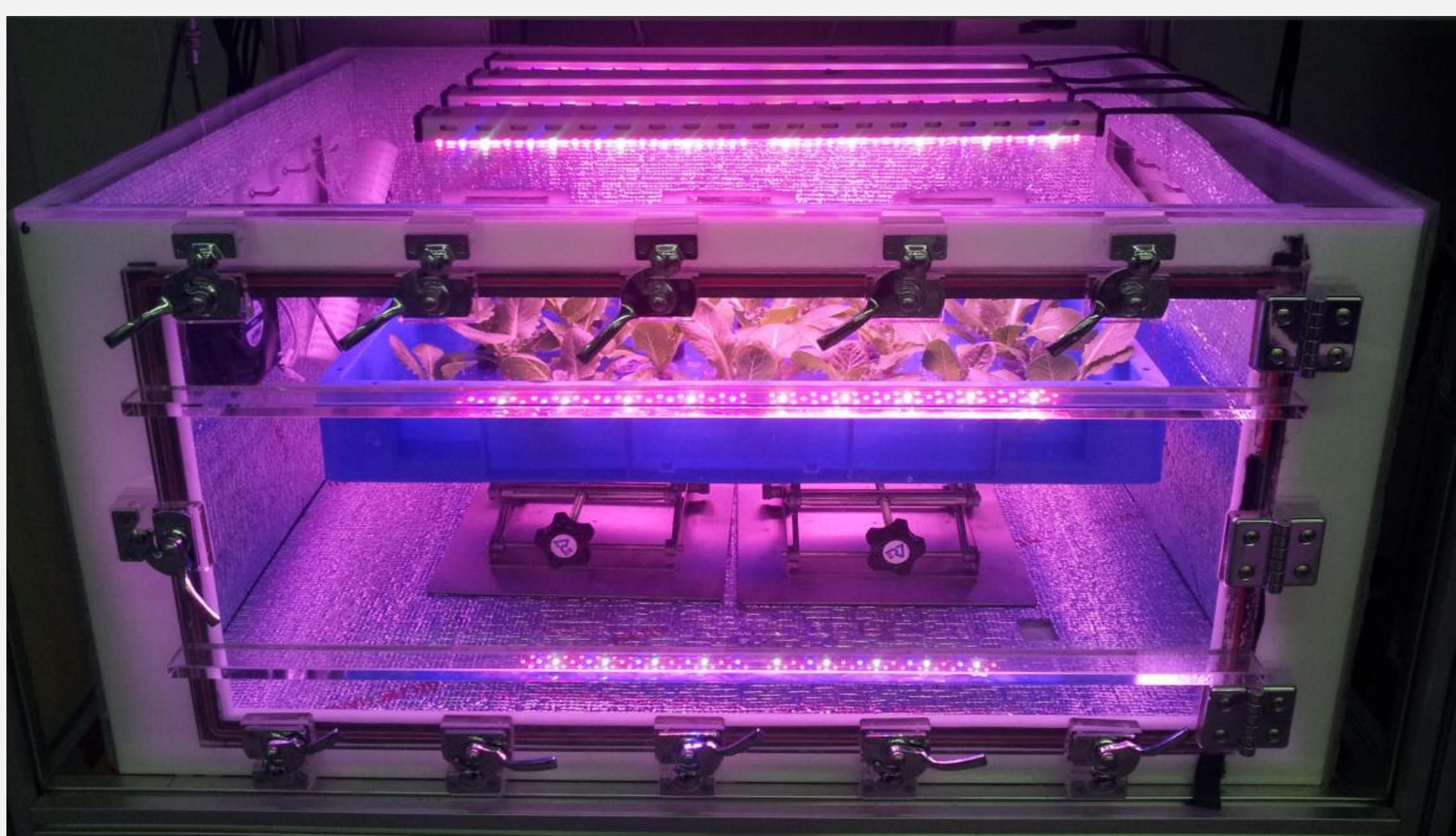
Fig. 1. Canopy photosynthetic rates of the lettuces were measured by using the acrylic chamber in which indoor temperature was controlled.
